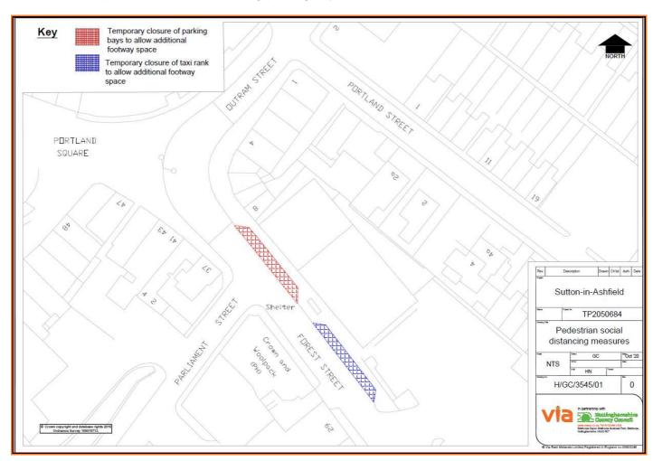
The roadspace will be reallocated for pedestrian use to facilitate appropriate social distancing within the town centre. As part of the work barriers will be erected to close the laybys to vehicles. The scheme will be introduced under a Temporary Traffic Regulation Order (TTRO) and it is anticipated that the measures may remain in place for a period of up to 12 months, the scheme will be monitored and reviewed as appropriate. Further information on the proposals is available:
