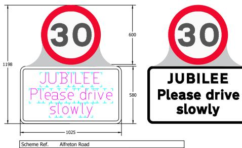
Sign B (terminal 30mph) 72.5 Sign Ref. x-height SIGN FACE Letter colour BLACK 1025mm WHITE Background Width Border BLACK Height 1198mm Material Class RA2 (12899-1:2007) Area 0.95m<sup>2</sup>
