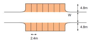
The width (W above) needed to access echelon or perpendicular spaces conveniently, depends on the width of the bay and the angle of approach. For a 2.4m wide bay, these values are typically:
