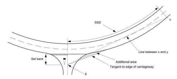
Where the line between points X and Y falls partially within the major road carriageway, an additional area shall be added to the visibility splay formed by drawing a line from X to a point tangential to the nearer edge of the major road running carriageway.
