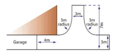
The area required for turning should not form part of the overall space required for parking. Driveway width subject to change, see Driveway widths above. Larger turning areas may be required if it is necessary to accommodate delivery vehciles.
