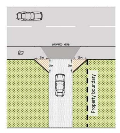
A vehicle emerging from a driveway at the back edge of a footway will require the driver to consider the possible presence of pedestrians. The absence of pedestrian visibility splays may encourage drivers to emerge more cautiously. Consideration should be given as to whether the absence of splays is appropriate, taking into account the frequency of vehicle movements, the amount of pedestrian activity, and the width of the footway.
